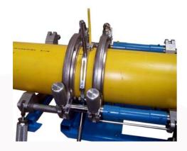
The pipes to be welded have to be clamped in such a way that the outside debeader will fit in between the clamping devices after completion of the welding process.
