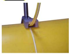
Rotate the outside debeader completely around the pipe, if necessary change-over the knurled grips.
