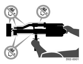
Always transport or store the hand extruder in such a way as to preclude any mechanical loads on the attachments.
