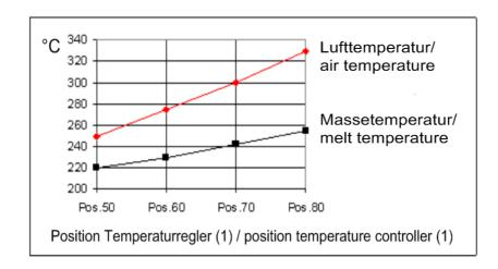
Check temperatures on the running extruder with an external thermometer after about 5 minutes.
